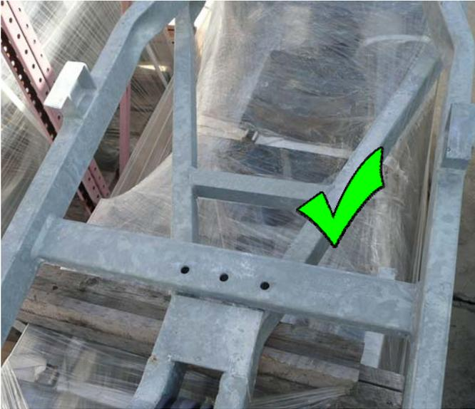
When using any kind of extended hoist mounting bracket, make sure the horizontal tube is 1-1/2x3" with a 3/16" thick wall.
